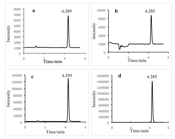
Fig. 2. Chromatogram of standard solution(a, 0.1 mg/L) and residual of pydiflumetofen in paddy water (b), soil (c), and rice straw (d).
